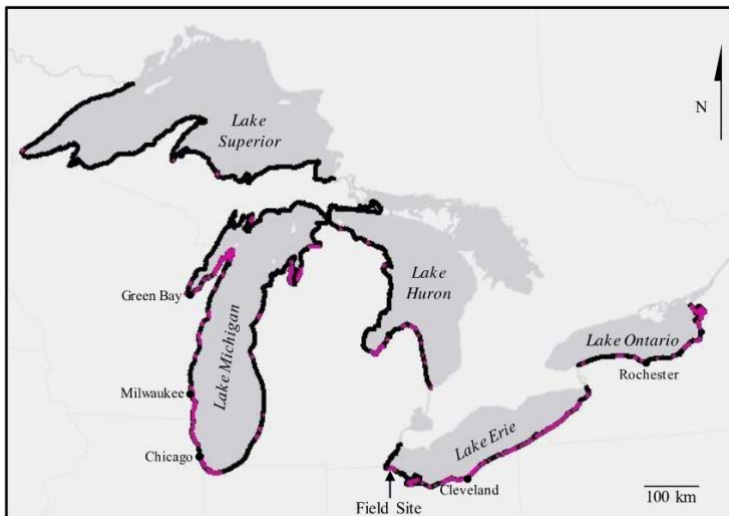
Figure 2 Vulnerability of Great Lakes to contaminant inputs from ground water. Bright color represent vulnerable areas.
