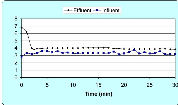
**Figure 4: Influent and effluent pH with slag #60, a bed depth of 2 in, a flow rate of 800 mL/min, and acidic influent.**
