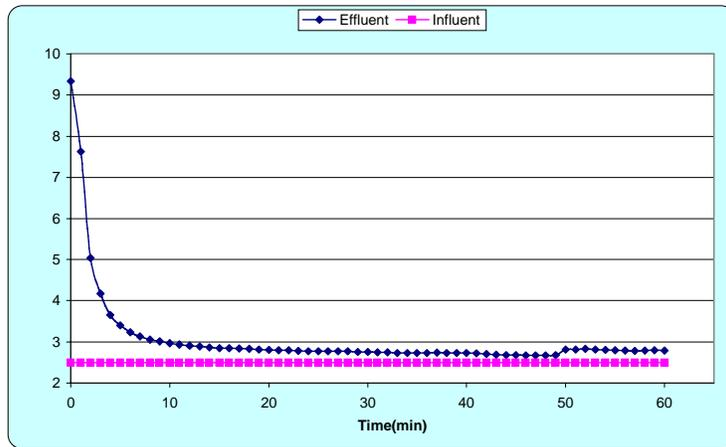
**Figure 8: Influent and effluent pH with slag #40, a bed depth of 1.5 in, a flow rate of 800 mL/min, and artificial AMD influent.**
