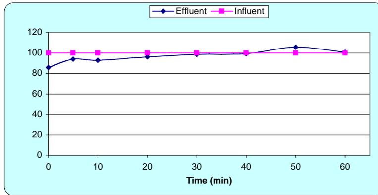
**Figure 10: Effluent and influent dissolved iron plotted against the time with slag #40, a bed depth of 1.5 in, a flow rate of 800 mL/min, and artificial AMD influent**
