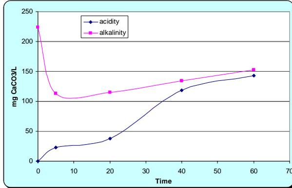
**Figure 7: Effluent alkalinity and acidity plotted against the time with slag #60, a bed depth of 2 in, a flow rate of 800 mL/min, and an acidic influent.**
