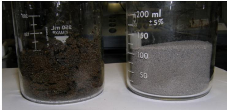
**Figure 14: Wet #40 slag from the fluidized bed reactor after 60 min of 800 mL/min flow with artificial AMD on left compared with fresh #40 slag on the right.**
