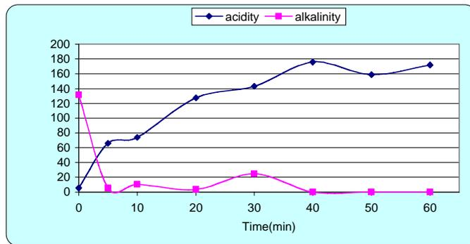
**Figure 12: Effluent alkalinity and acidity plotted against the time with slag #40, a bed depth of 1.5 in, a flow rate of 800 mL/min, and artificial AMD influent**
