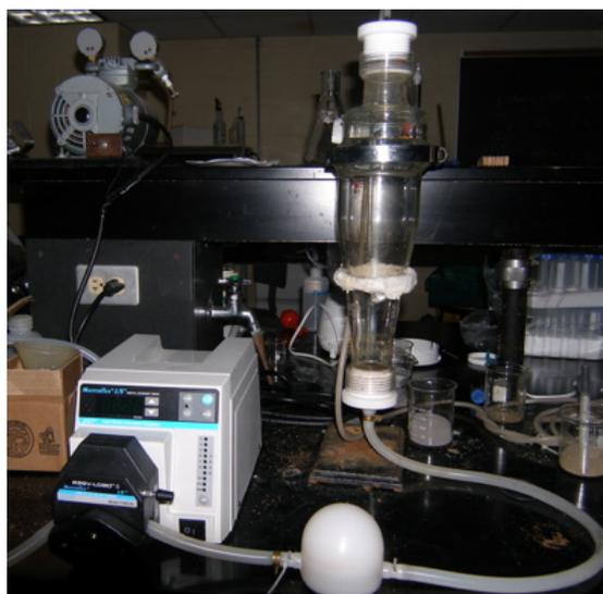
**Figure 2: Peristaltic pump and fluidized bed reactor**
