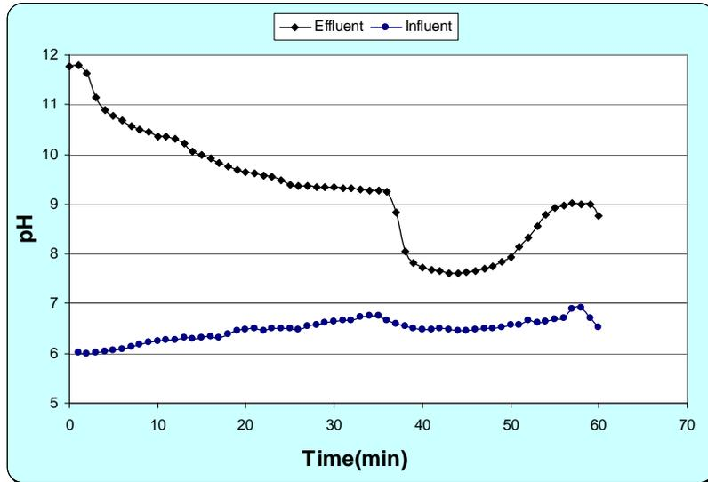
**Figure 6: Influent and effluent pH with slag #60, a bed depth of 2 in, a flow rate of 800 mL/min, and acidic influent.**
