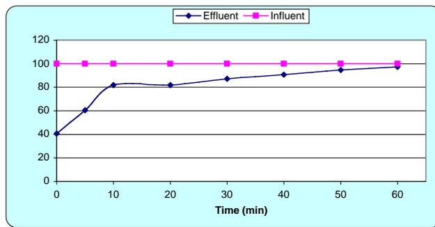
**Figure 13: Effluent and influent dissolved iron plotted against the time with slag #40, a bed depth of 1.5 in, a flow rate of 800 mL/min, and artificial AMD influent**
