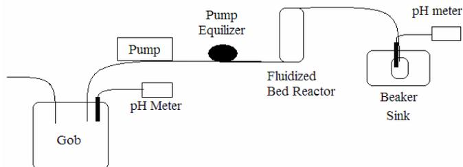
**Figure 1: Fluidized Bed Reactor Setup**
