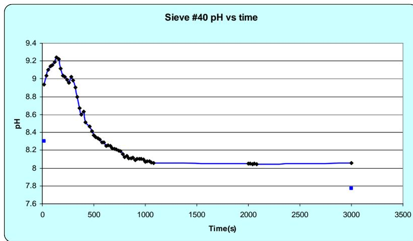
**Figure 3: Effluent pH with a 1 in layer of # 40 slag, a flow rate of 800 mL/min, and tap water.**
