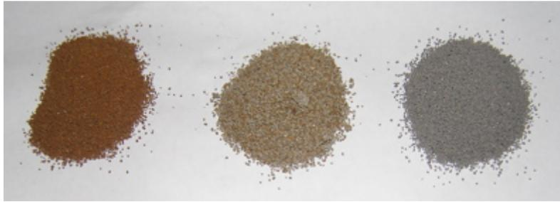
**Figure 15: Dry #40 slag from the fluidized bed reactor after 60 min of 800 mL/min flow with artificial AMD (left), dry #40 slag from the fluidized bed reactor after 60 min of 800 mL/min flow with gob leachate (middle), and fresh #40 slag (right).**
