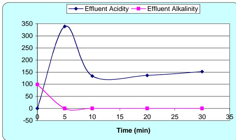
**Figure 5: Effluent alkalinity and acidity plotted against the time with slag #60, a bed depth of 2 in, a flow rate of 800 mL/min, and an acidic influent.**
