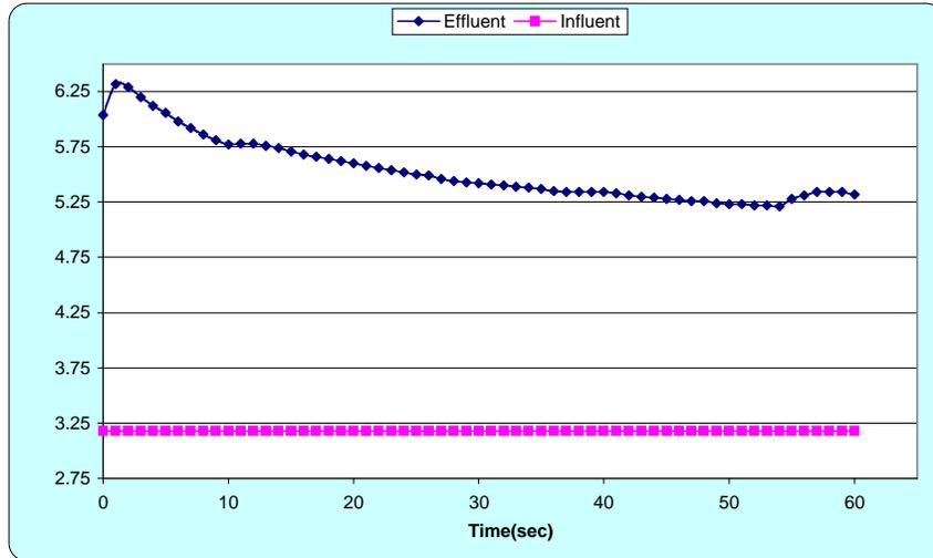
**Figure 11: Influent and effluent pH with slag #40, a bed depth of 1.5 in, a flow rate of 800 mL/min, and artificial AMD influent.**
