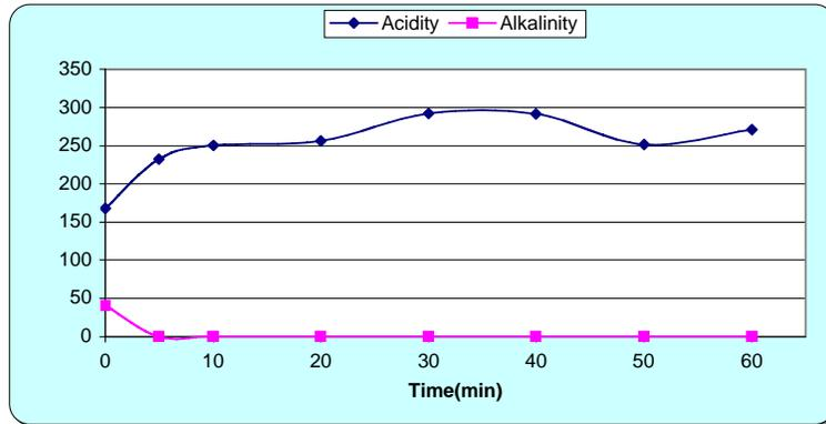
**Figure 9: Effluent alkalinity and acidity plotted against the time with slag #40, a bed depth of 1.5 in, a flow rate of 800 mL/min, and artificial AMD influent**
