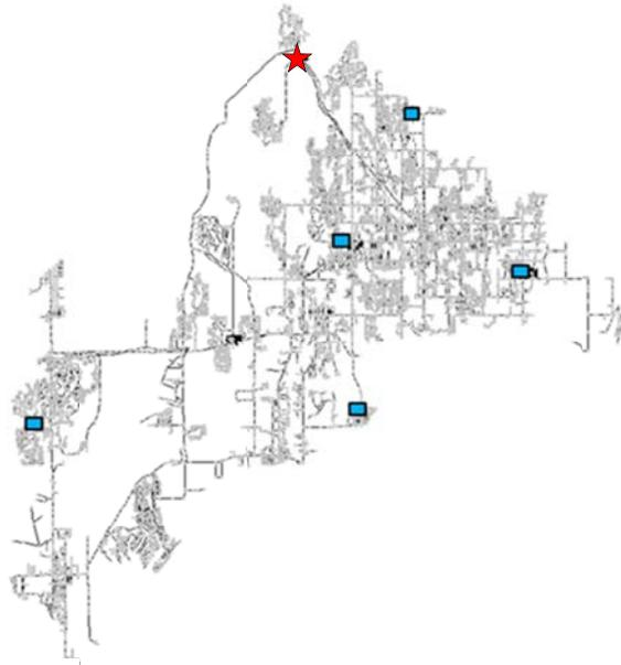
Figure 7. Layout of the large test network with the injection location indicated by a star and the five sensor locations indicated by the rectangles.
