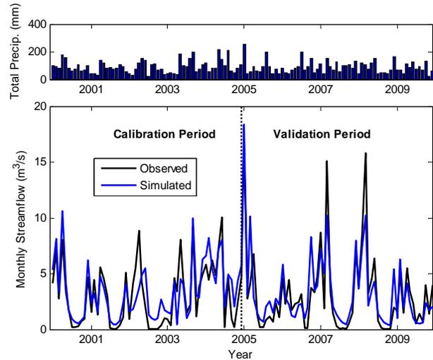
**Figure 2:** Flow calibrated SWAT Model for UBWC Watershed. Comparison of mean monthly observed streamflow to simulated streamflow at USGS Gauge 03228300 (Sunbury, OH) for the model calibration and validation periods of 2000-
