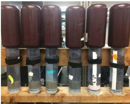
Figure 1. Experimental setup to determine the phosphorous sorption capacity of water treatment plant residuals.
