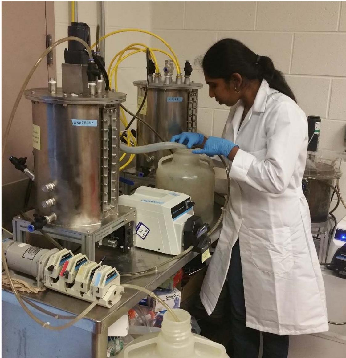
Figure. A graduate student (Brindha Murugesan, M.S. candidate) is optimizing a bench-scale membrane bioreactor system with the carbon nanotube composite membrane for efficient removal of nitrogen and phosphorus from municipal wastewater.
