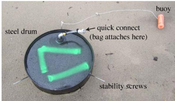
**Figure 2:** Photograph of a Lee-type seepage meter used by PI Sawyer's laboratory.
