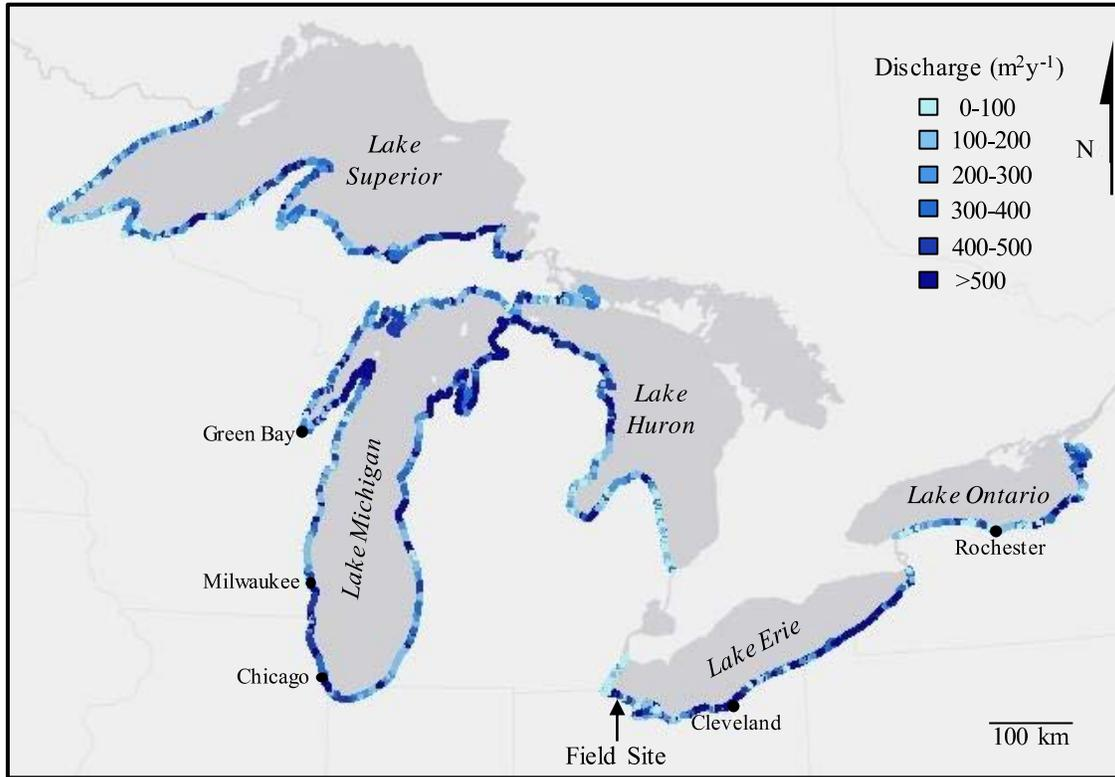
**Figure 3:** Direct ground water discharge to the Great Lakes. Discharge rates are high along the eastern and central sections of Lake Erie.
