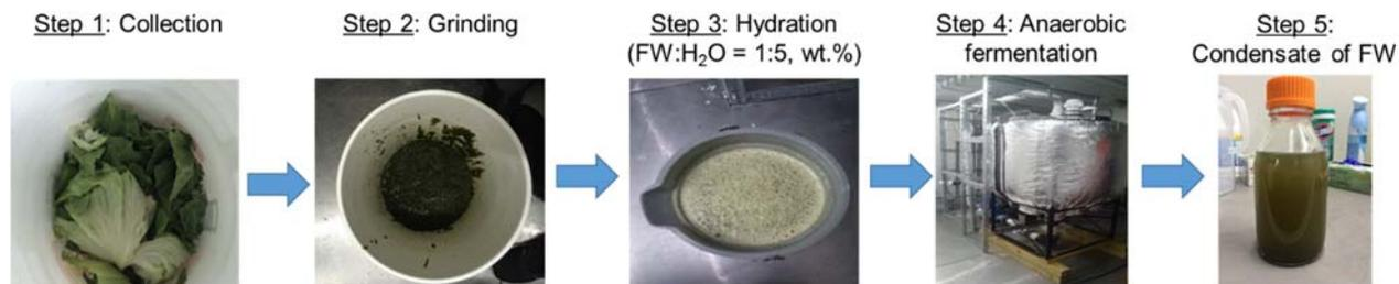
**Figure 1.** Schematic diagram of an anaerobic fermentation process for production of CFW.
