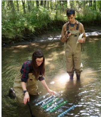
Figure 1 Dr. Costello's students installing trace metal diffusing substrates in stream.
