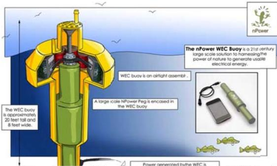
**Figure 1** The nPower® Personal Energy Generator (PEG), which can be used to recharge mobile devices by harvesting the kinetic energy generated from walking (inset), and a schematic of a proposed nPower® Wave Energy Converter (WEC) encased in an airtight buoy.
