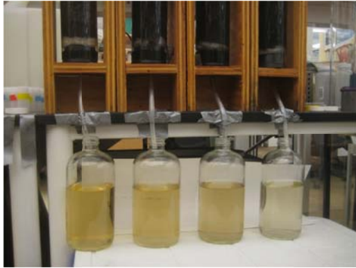
Figure 1 Leachate from laboratory columns of green roof growing media with varying amounts of biochar ranging from no biochar (left) to high biochar (right). Note the reduction in color in the water is due to biochar binding organic matter which minimizes its elution.
