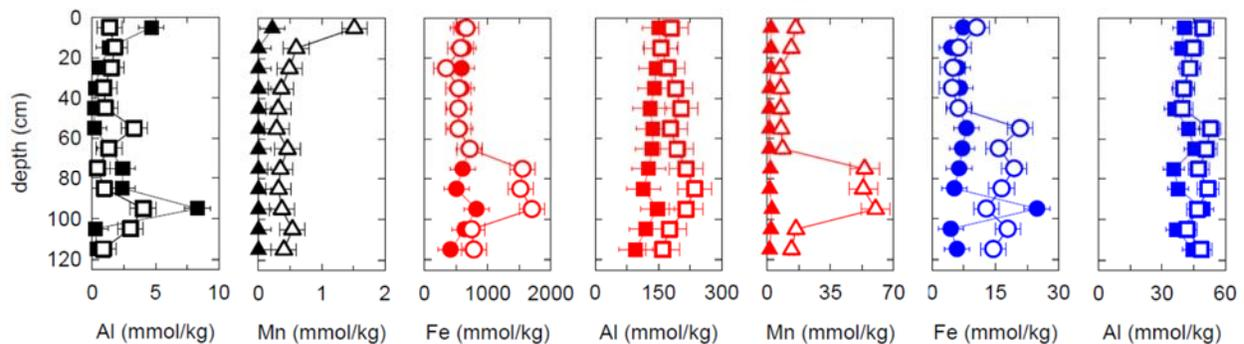
**Figure 2** Sequential extraction data for Fe (circles), Al (squares), and Mn (triangles) from the highwall (closed symbols) and mine tailings (open symbols) soil cores. The three fractions are exchangeable (black), reducible (red), and oxidizable (blue).
