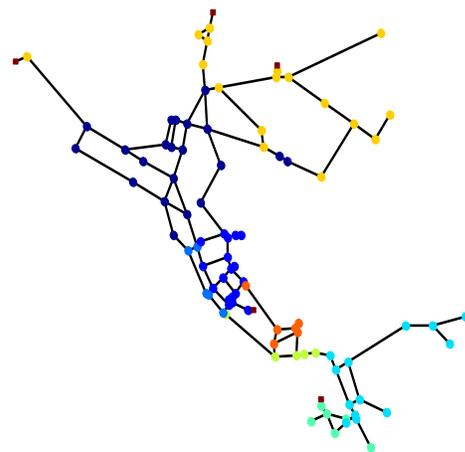
**Figure 2.** Results of the clustering algorithms applied to a small test case network. The consumer nodes (circles) have been clustered into eight groups of nodes with similar hydraulic impacts.
