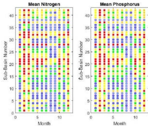
**Figure 2** Monthly Mean Nitrogen and Phosphorus Load among 42 Subbasins and 12 Months in UBWC. Vertical features indicate times of year of interest whereas horizontal features indicate areas within the catchment that consistently contribute to NPS. Red are top six contributors.
