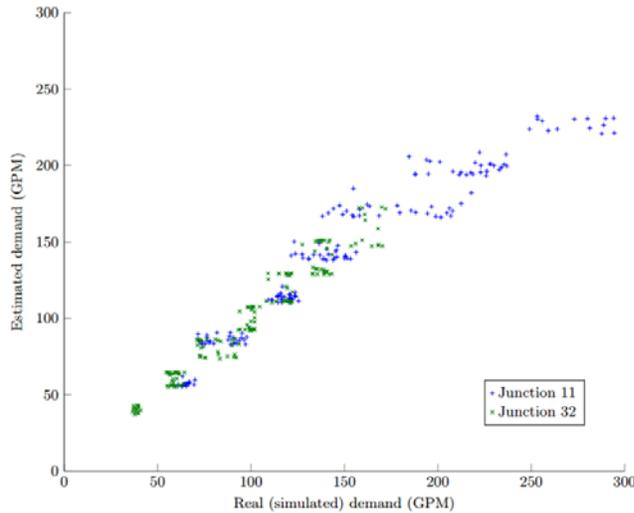
**Figure 1** Scatter plot of the estimated (Y axis) versus the “real” (X axis) demands for best and worst performing consumer nodes for one-week time span. Junction 11 – blue plus signs, Junction 31 – green crosses.
