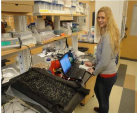
Figure 1 Caitlin Shaw overseeing plot and scale setup for continuous recording of weight changes due to evaporation from biochar-amended vegetated roof substrate.
