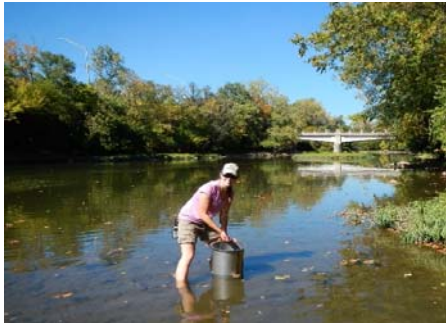
Figure 1. Student Ellen Comes uses McNeil sampler on the Olentangy River to characterize riverbed sediment.
